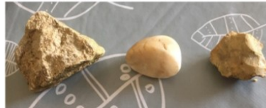
1. SANDSTONE BROWN AND YELLOW COLOUR ROUGH FINISH GRANULAR 2. QUARTZ WHITE AND YELLOW COLOUR SMOOTH FINISH SHINY 3. FLINT YELLOW AND BROWN COLOUR SHARP EDGES SHINY
